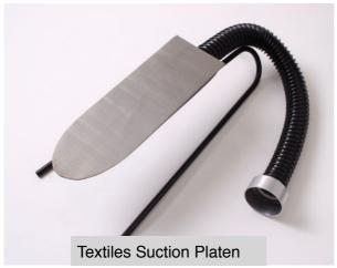
The range of RH Suction Platens are mini suction tables for use when the suction table has to be brought to the object, such as a book, clothing or canvas painting on a stretcher. It is used for cleaning, holding and pressing paper and textiles, pulp filling of paper, cold patch lining of canvas paintings and textiles or where an even suction is required on a small flat surface.
