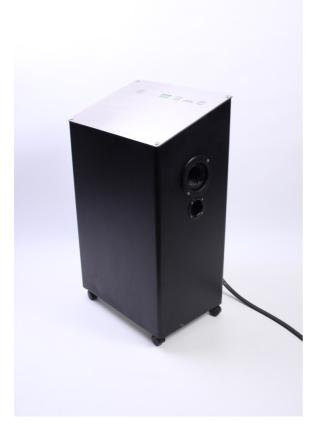
The RH Suction Unit is designed for use with the RH Suction Table Worktop and the RH Suction Platen. It stands 950 mm high, 540 mm wide and 375 mm deep and rolls on 50 mm castors. The outer casing of the unit is matt black anodised aluminium and the control panel on the inclined top is stainless steel. The control panel is completely flush and sealed to all solvents used in conservation.
