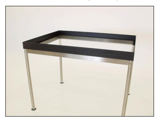
The RH Washing Tray is designed for washing paper and textiles. It is constructed of 80 mm high matt black anodised aluminium sides, 6 mm thick safety glass base and a stainless steel magnetic drainage valve in one corner. A screw-in flexible drain hose is also supplied.
